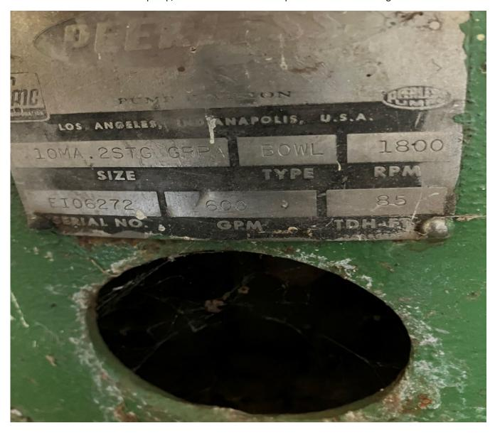
• **Motor-** We will also need a motor that will match and run the pump above, that meets the specifications of the data plate pictured below.
